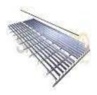
**SkyFuel** was awarded a grant by the U.S. Department of Energy (DOE) to develop its advanced Concentrating Solar Power system known as the **Linear Power Tower** for utility-scale solar thermal power plants. LPT is a high-temperature linear Fresnel system with molten salt storage. The diagram at left looks like a grill for an air conditioner, but it actually shows a football pitch-sized array of solar mirrors.
